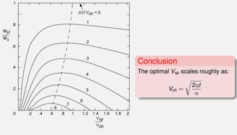
Payload fraction vs.  $V_{sp}$  for  $\Delta V \ll V_{ch}$
