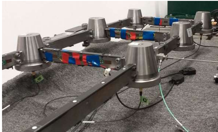
Figure 1: Demonstration stand with six lockable joints
