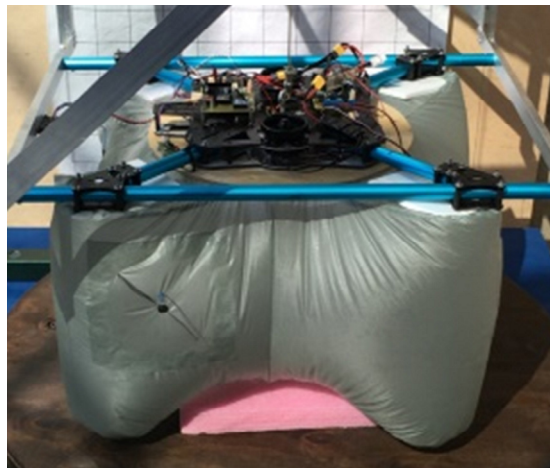
Figure 2. Complete AdBag system with a target-shaped airbag, prepared for drop tests
