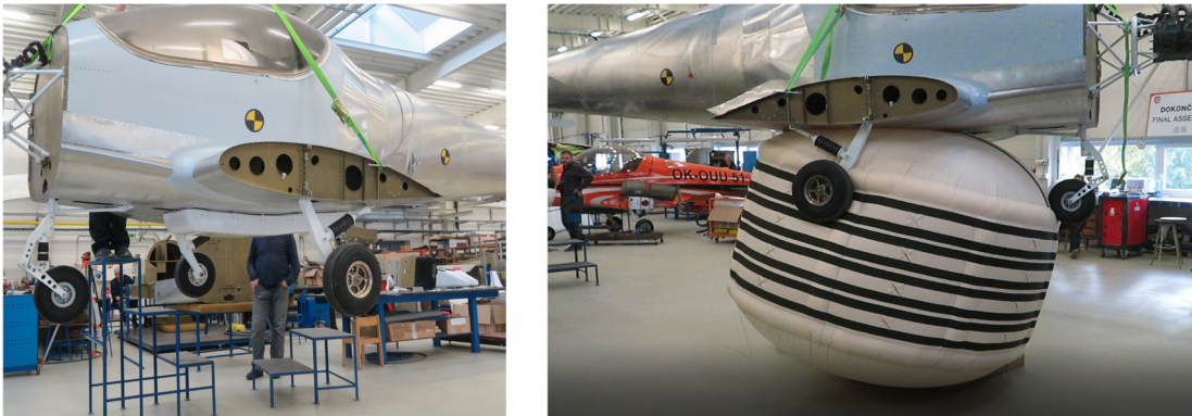
Figure 7. The Softland system installed on the aircraft: a. airbag in the closed state, b. airbag in the open state
