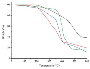
Figure 4. Thermograms of  $PT6N(EtOH)_2$  (black line),  $PT6buP^+Br^-$  (green line),  $PTO6buP^+Br^-$  (blue line), and  $P(EDOT-MeO6buP^+Br^-)$  (red line).
