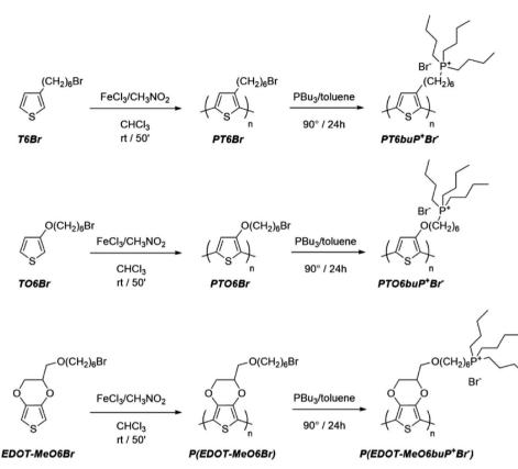
Scheme 1. Synthetic routes to obtain the CPE interlayers (PT6buP<sup>+</sup>Br<sup>-</sup>, PTO6buP<sup>+</sup>Br<sup>-</sup>, and P(EDOT-MeO6buP<sup>+</sup>Br<sup>-</sup>)).
