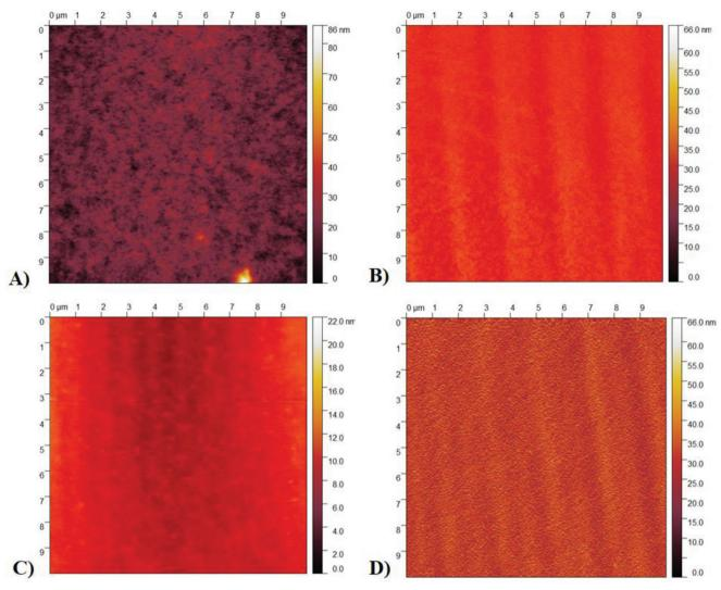
Figure 9. AFM topography images of A) PT6N(EtOH)<sub>2</sub> layer and of PT6N(EtOH)<sub>2</sub> after spray-coating of B) PT6buP<sup>+</sup>Br<sup>-</sup>, C) PTO6buP<sup>+</sup>Br<sup>-</sup>, and D) P(EDOT-MeO6buP<sup>+</sup>Br<sup>-</sup>) outer layer.
