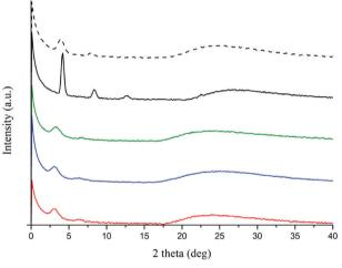
**Figure 6.** X-ray diffractograms of PT6N(EtOH)<sub>2</sub> not annealed (dashed line) and annealed (black line), PT6buP<sup>+</sup>Br<sup>-</sup> (green line), PT06buP<sup>+</sup>Br<sup>-</sup> (blue line), and P(EDOT-MeO6buP<sup>+</sup>Br<sup>-</sup>) (red line).
