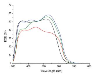
Figure 11. EQE spectra of the tested devices:  $PT6N(EtOH)_2:C_{60}$ -Ser without (red line) and with interlayer:  $PT6buP^+Br^-$  (green line),  $PTO6buP^+Br^-$  (blue line), and  $P(EDOT-MeO6buP^+Br^-)$  (black line).
