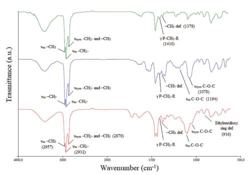
Figure 3. FT-IR spectra of PT6buP<sup>+</sup>Br<sup>-</sup> (green line), PTO6buP<sup>+</sup>Br<sup>-</sup> (blue line), and P(EDOT-MeO6buP<sup>+</sup>Br<sup>-</sup>) (red line).
