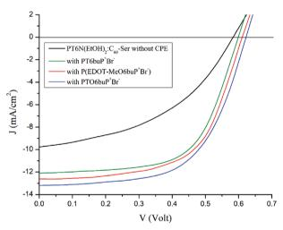
**Figure 7.** Current density–voltage (J/V) for the best-performing cells tested under AM 1.5 one-sun illumination.
