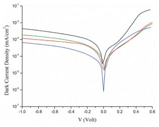
**Figure 8.** Semilogarithmic current density versus voltage curves of the prepared devices measured in the dark:  $PT6N(EtOH)_2$  (black line),  $PT6buP^+Br^-$  (green line),  $PTO6buP^+Br^-$  (blue line), and  $P(EDOT-MeO6buP^+Br^-)$  (red line).
