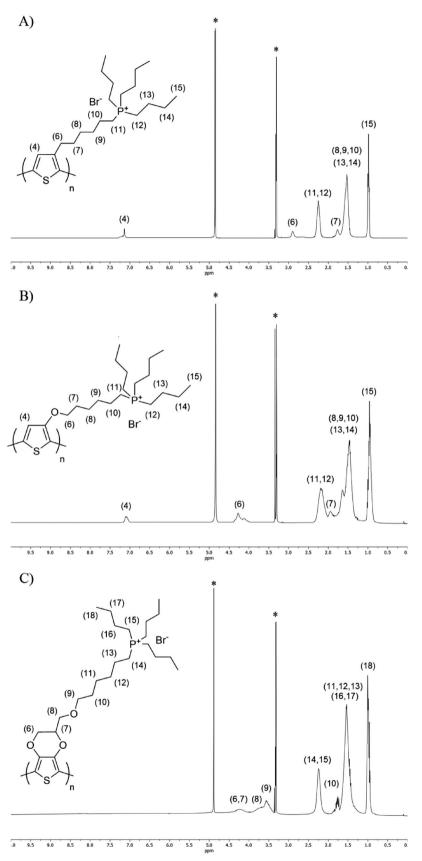
Figure 2. <sup>1</sup>H-NMR spectra of A) PT6buP<sup>+</sup>Br<sup>-</sup>, B) PTO6buP<sup>+</sup>Br<sup>-</sup>, and C) P(EDOT-MeO6buP<sup>+</sup>Br<sup>-</sup>). Asterisk: solvent resonance (CD<sub>3</sub>OD).
