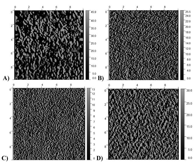
**Figure 10.** AFM phase images ( $10 \times 10 \mu$ m; z-scale: in degrees) of A) PT6N(EtOH)<sub>2</sub> layer and of PT6N(EtOH)<sub>2</sub> after spray-coating of B) PT6buP<sup>+</sup>Br<sup>-</sup>, C) PTO6buP<sup>+</sup>Br<sup>-</sup>, and D) P(EDOT-MeO6buP<sup>+</sup>Br<sup>-</sup>) outer layer.
