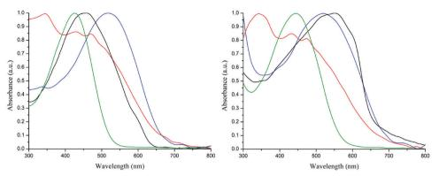
Figure 5. Normalized UV-vis spectra of polymers in methanol solution (left) and in film (right) from MeOH: PT6N(EtOH)<sub>2</sub> (black line), PT6buP<sup>+</sup>Br<sup>-</sup> (green line), PT06buP<sup>+</sup>Br<sup>-</sup> (blue line), and P(EDOT-MeO6buP<sup>+</sup>Br<sup>-</sup>) (red line).
