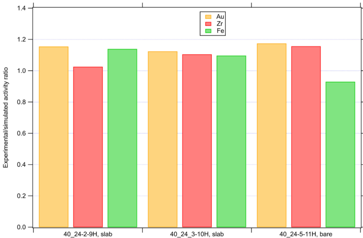
Fig. 4b. the measured over calculated activities of Au 0.1%-Al (IRMM-530), zirconium, and iron foils irradiated in Pos. 2 of the No. 17 channel.
