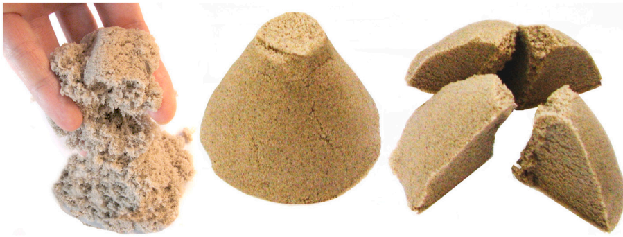
Fig. 1. Mixture of a 98% of fine sand and 2% coating called kinetic sand.
