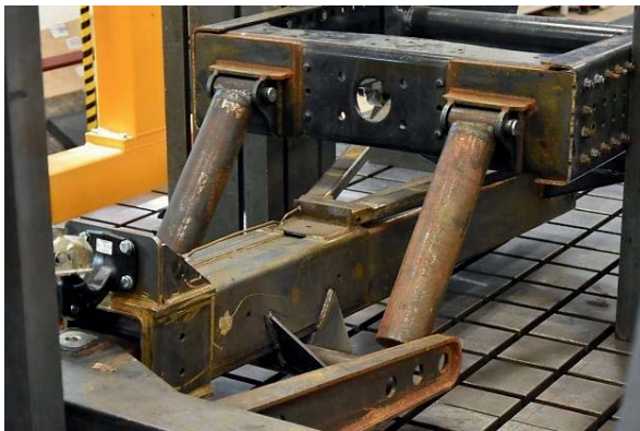
Figure 6. Swing frame (material: S235 steel) with a fork, actuators and A50-X class ball coupled with a testing stand station.
