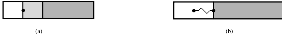
Fig. 5. Different approaches for modelling the DEM-BEM interface: (a) coupling the displacement of the DE particle centre with BE end-node displacement (lighter grey indicates overlap, reason why the particle must have half the mass) and (b) coupling through an interaction model between the DE particle and the BE region.
