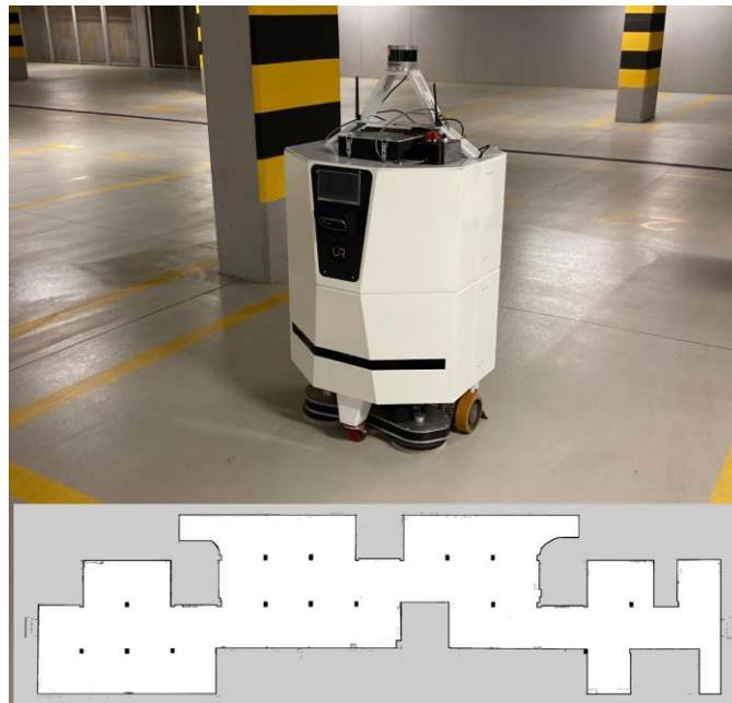
Figure 1. The cleaning robot with a 2D static map of a garage to be cleaned.
