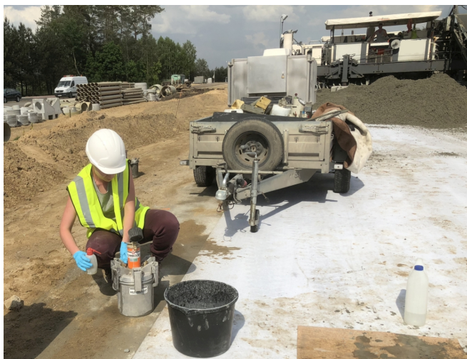
Fig. 3. Field measurements of air content and air void size distribution using SAM apparatus
