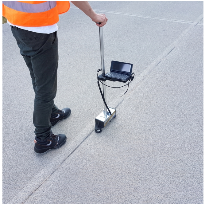
Fig. 8. Longitudinal evenness measurement with a Dipstick.
