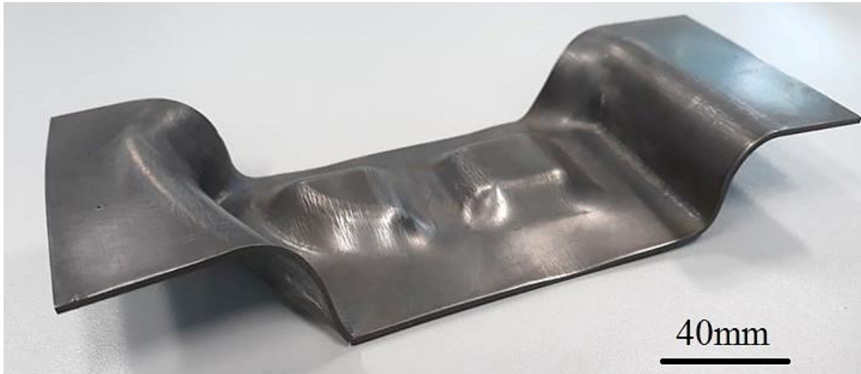
Fig. 14 TC4 wing stiffener formed by FAST (heating temperature 900 °C)
