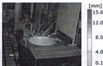
Fig. 4. Distributions of the resultant vectors in the SUV wheel under the loading of 11kN for the tire
