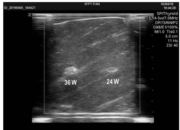
Fig. 8. Ultrasound image of the axial section ( yz ) of the tested tissue sample placed in the cylindrical chamber after its exposure at the front and back to two coaxial HIFU beams with the acoustic power of 24 W and 36 W.
