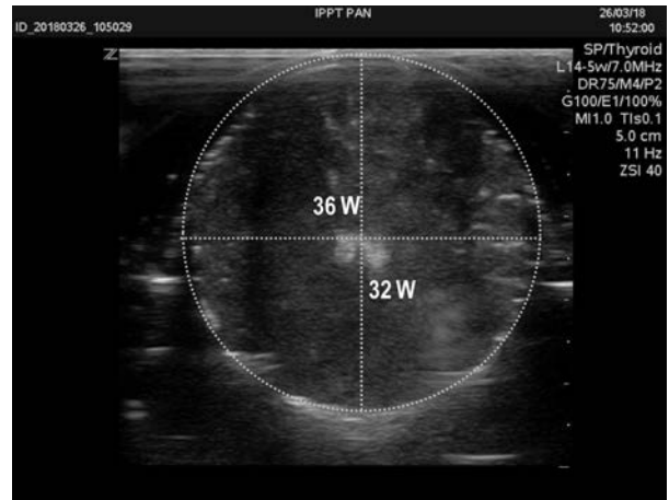
Fig. 6. Ultrasound image of the radial section ( xy ) of the tested tissue sample placed in the cylindrical chamber after its exposure to two parallel, spaced by 4 mm, HIFU beams with the acoustic power of 32 W and 36 W. The section at a focal plane of the beams is shown.
