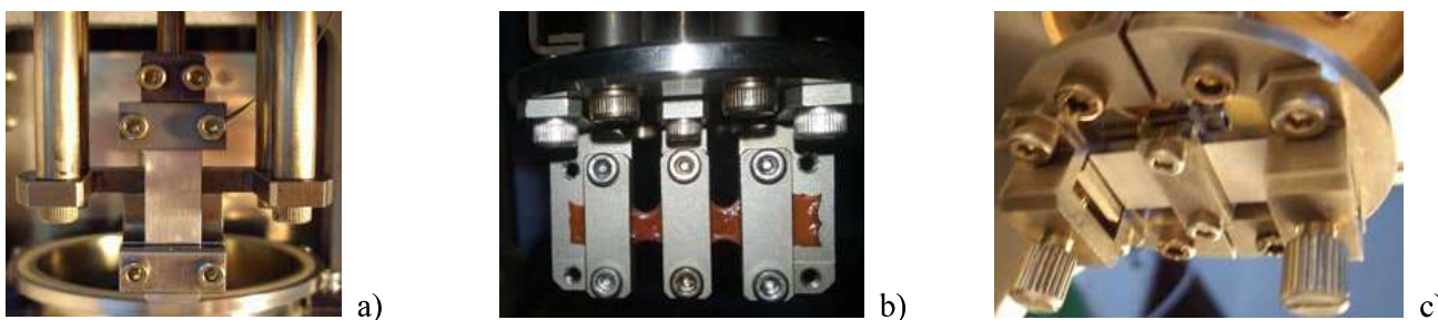
Figure 1. Fixtures used in the DMA experiments: tension (a), shear (b), bending (c).
