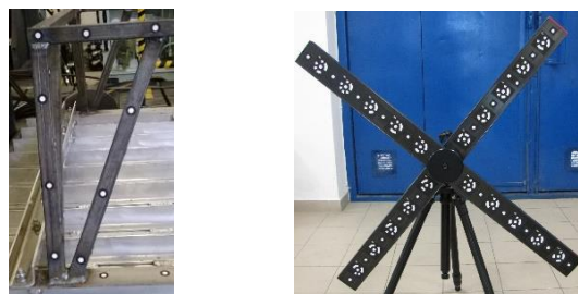
Fig. 1. DIC technique details: distribution of markers for measurements and calibration cross
