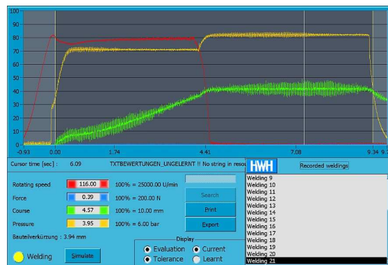
Fig.2. The graph of friction welding conditions as a function of time (image from computer monitor).
