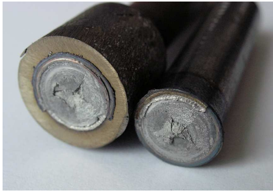
Fig.4. Fracture surfaces of bonded elements.
