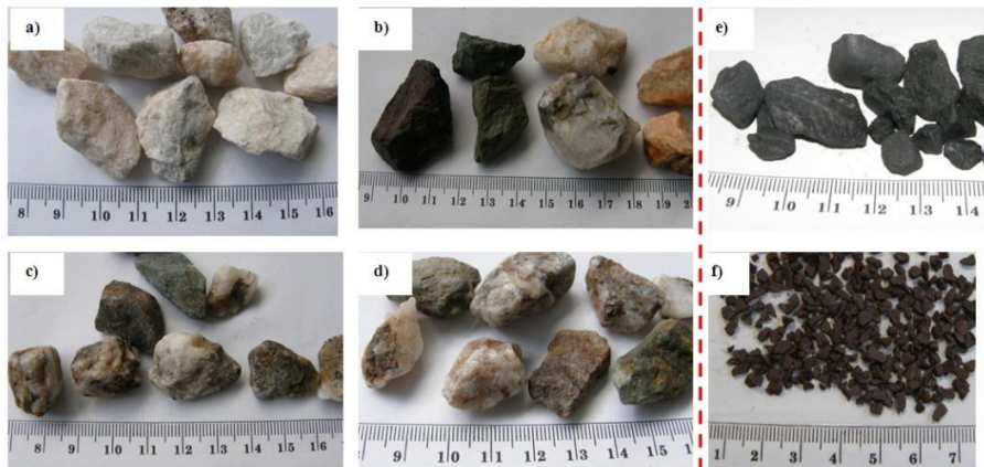
Fig. 1. Photographs of barite grains(a) B1 from Germany; (b) B2 from Czech Republic(c) B3 from Poland ; (d) B4 from Czech Republic, (e) magnetite from Sweden; (f) hematite from Morocco.
