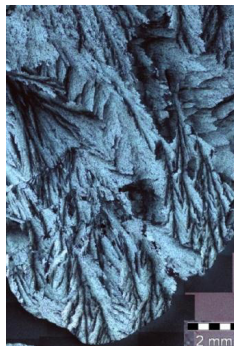
Fig. 2. Radial growths of barite B2 crystals, after XPL (scale bar = 2 mm).
