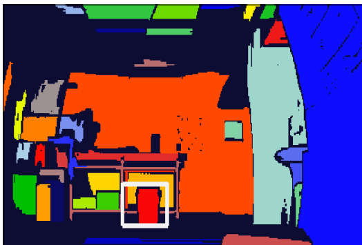
Figure 4. Areas A_i resembling continuous objects in real space (for each area, the real distance between neighbouring pixels is smaller than 5cm). The white rectangle denotes the region which has been recognized by the Haar classifier as a wastebasket.
