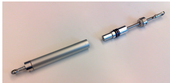
Figure 2.1: Schematic of the pneumatic impact energy absorber with the reaction force value control circuit (left) and the disassembled absorber (right)
