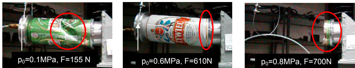
Figure 5.2: Deformation of the beverage can with internal pressure: a) 0,1 MPa, b) 0,6 MPa, c) 0,8MPa
