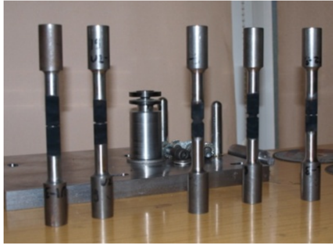
Figure 4.26: The picture of manufactured specimens, the notched zones are blackened for observation with use of the thermographic camera.
