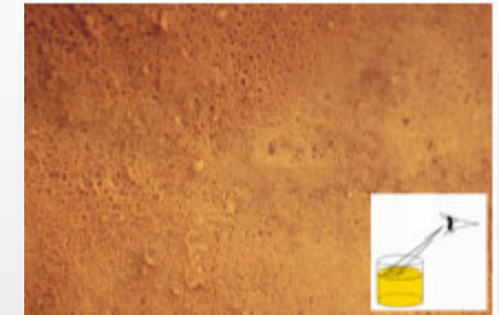
Flow regimes in sand-water mixtures under seepage conditions
