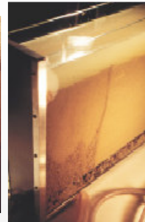
Filter instability (left) and air bubbles trapped in horizontal barriers of very fine particles
