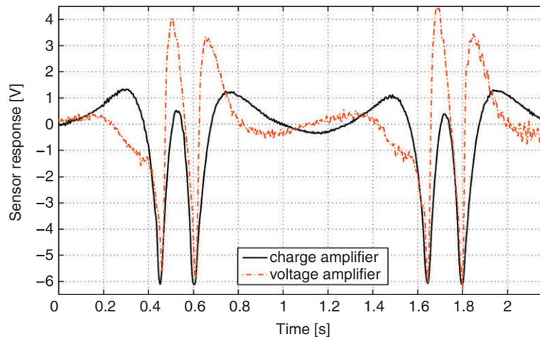
Figure 10. Performance of voltage and charge amplifiers exemplified by differences in time signals.
