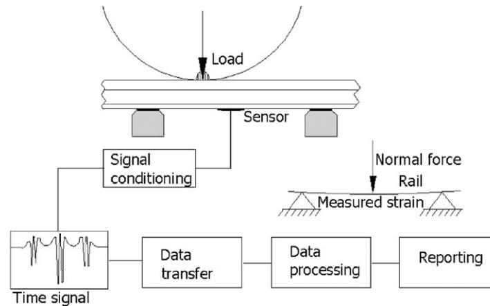
Figure 3. Scheme of data acquisition and processing for the proposed WIM system.
