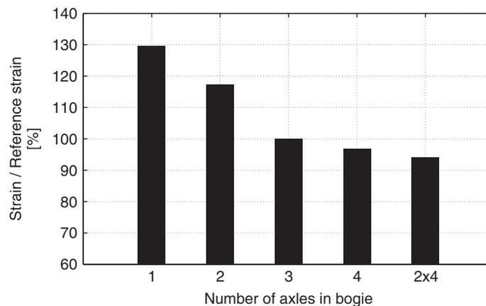
Figure 16. Rail strains as a function of load distribution.
