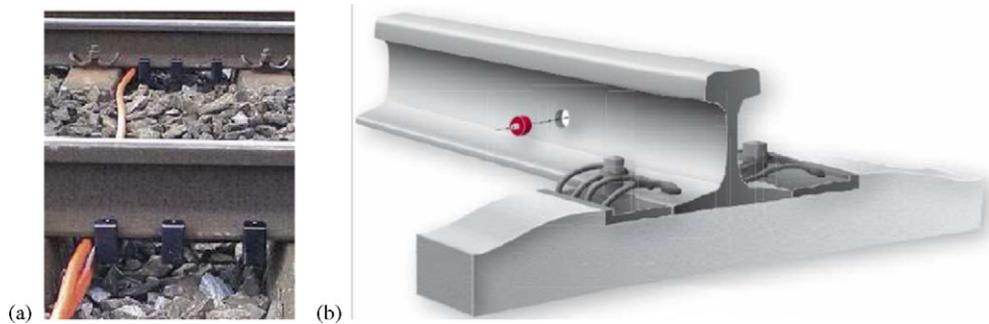
Figure 1. Example of WIM applications for railways: (a) fibre optic sensors TagMaster [18] and (b) intrusive quartz sensor Kistler [19].
