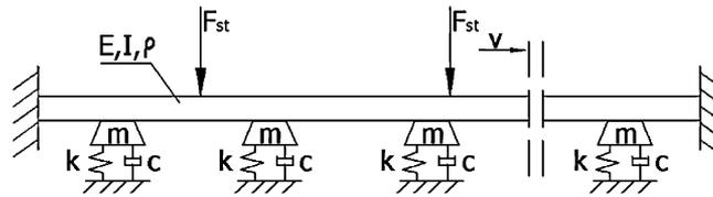
Figure 12. Model of the rail–sleeper–ground interaction.
