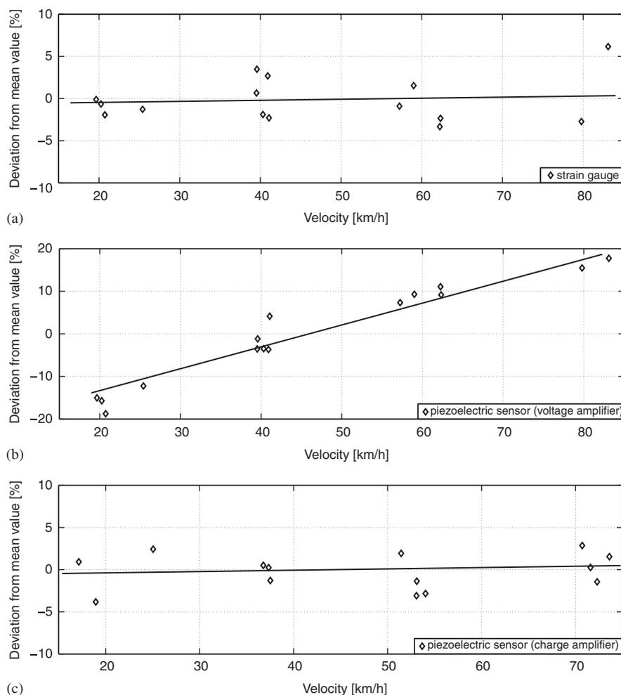
Figure 11. Velocity effect on the measured signal: (a) strain gauge; (b) piezoelectric sensor with voltage amplifier; and (c) piezoelectric sensor with charge amplifier.
