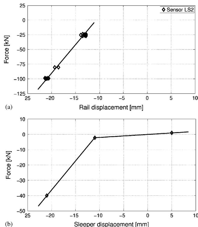
Figure 13. Force–displacement characteristic of the track: (a) measured *in situ* and (b) used in the model.
