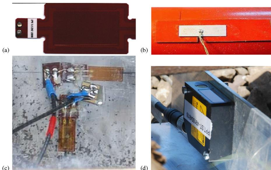
Figure 5. Sensors used in experimental tests: (a) piezoelectric fibre composite *PFC* sensors; (b) piezoceramic sensors based on the PZT-7 material; (c) half-bridge configuration of strain gauges; and (d) laser displacement sensor.
