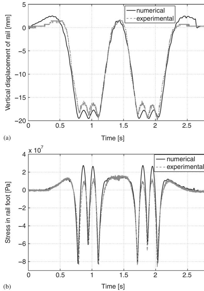
Figure 14. Numerical vs experimental results: (a) vertical displacements of the rail and (b) stresses in the rail foot.
