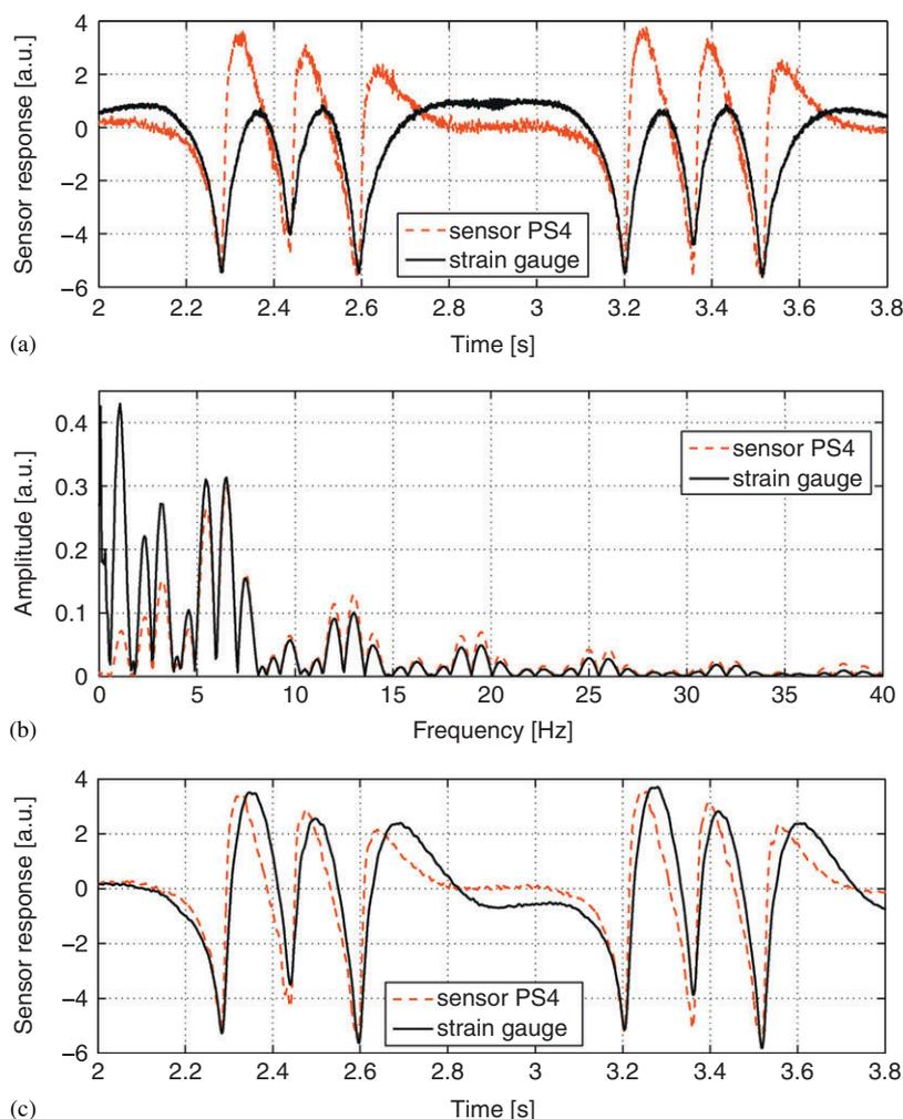
Figure 9. Signals from two types of sensors due to the passage of the *ET-22* locomotive: (a) direct measurements in the time domain; (b) spectra in the frequency domain; and (c) filtered signals in the time domain.
