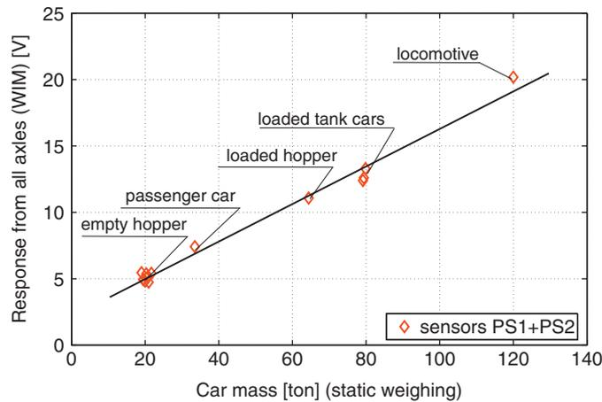
Figure 7. Voltage–mass relationship obtained on the basis of calibration from static weighing.
