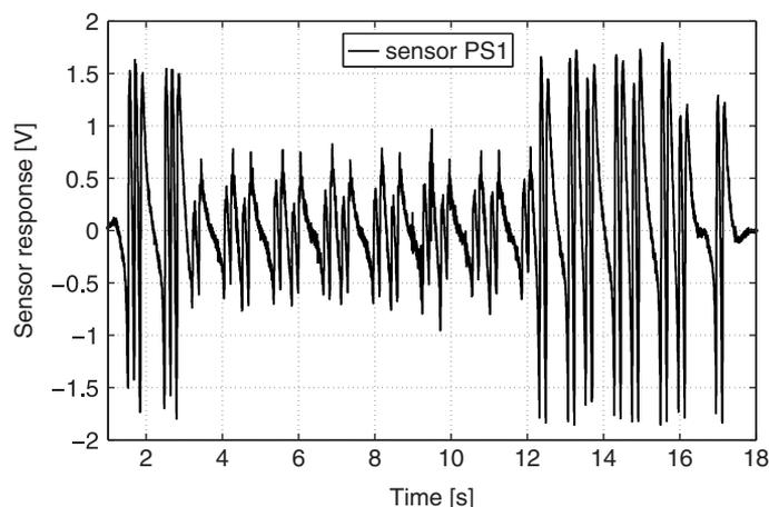
Figure 6. Time signal from the piezo-sensor as a response to passage of a freight train.
