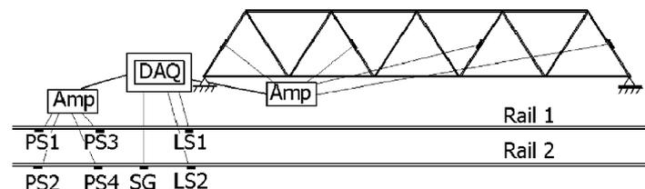
Figure 4. Components of the proposed WIM system during *in situ* tests: PS1, PS2, PS3, PS4, piezoelectric sensors; SG, strain gauge; LS1, LS2, laser sensors recording displacements; AMP, amplifier; DAQ, data acquisition unit.
