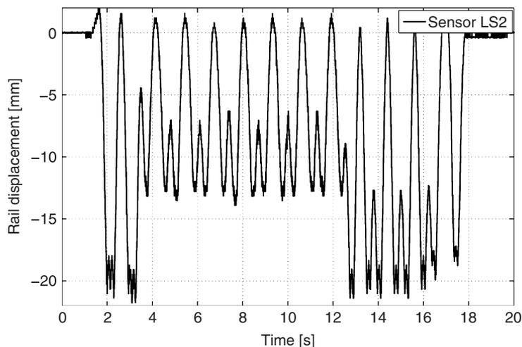
Figure 8. Vertical displacements of rail recorded by the laser sensor.
