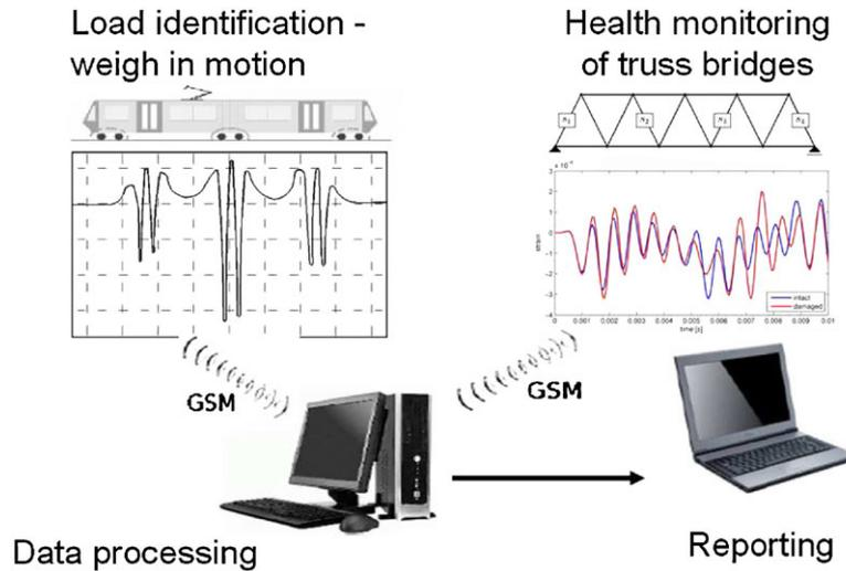
Figure 2. General scheme of the system for SHM of truss bridges integrated with the rail-WIM system.
