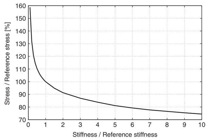
Figure 15. Rail stresses as a function of support stiffness.
