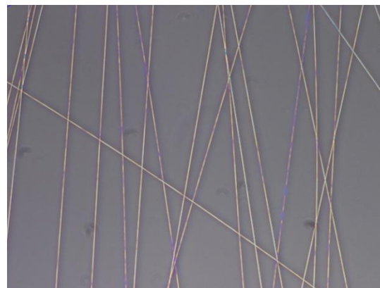
PLA 15KV fibers seen at optical microscope at 10x
